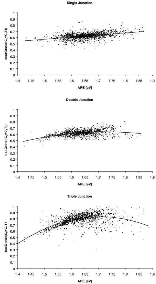
**Figure 4.** The purely spectral influence of APE on device efficiency.
