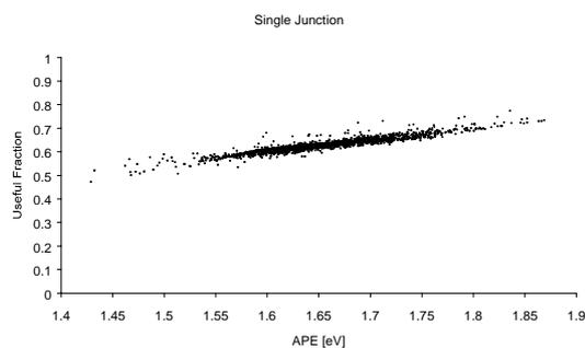
**Figure 1.** Relationship between average photon energy and useful fraction for a single junction a-Si device.
