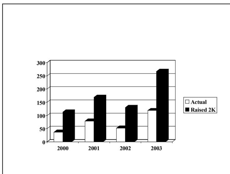
**Figure 4: Cooling degree days for Royston at actual and (theoretical) raised temperatures**
