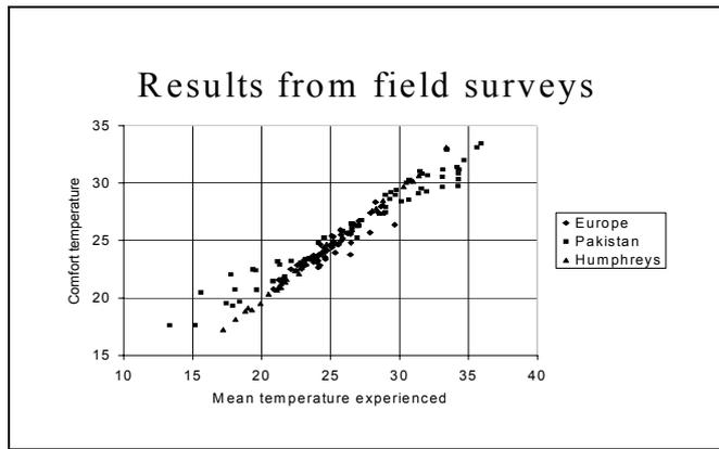
**Figure 2: comfort temperatures over a range of outdoor temperatures**
