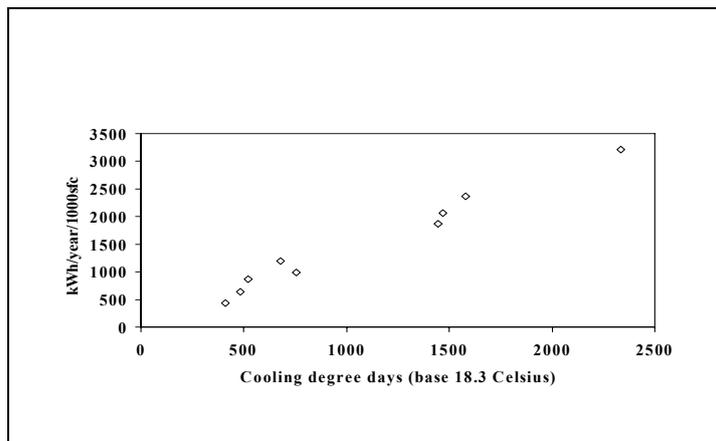
**Figure 3: electricity consumption due to air-conditioning in relation to cooling degree days**
