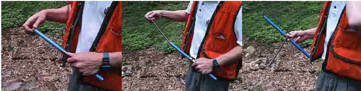
Figure 3. How to assemble an increment borer
