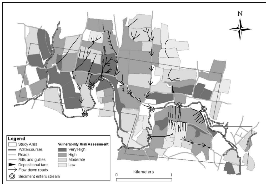
Fig. 6. Risk of damage to road or river downslope of field in Sample Site 2.
